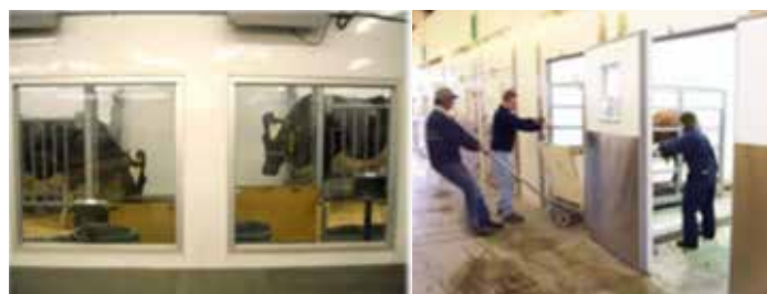
Environmental chambers used to measure enteric methane emissions at (left) the Dairy and Swine Research and Development Centre, Sherbrooke, Québec and (right) the Lethbridge Research Centre, Alberta.
