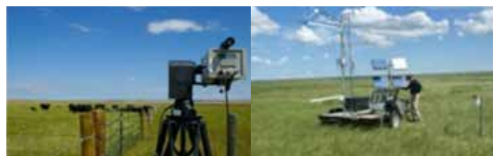
CO 2 exchange above pasture and enteric CH 4 emissions measured on grazing cattle using micro-meteorological techniques at the Lethbridge Research Centre.
