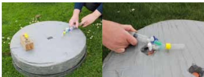
Chamber deployment. Insulated cover with water trough base (left); Headspace sampling (right).
